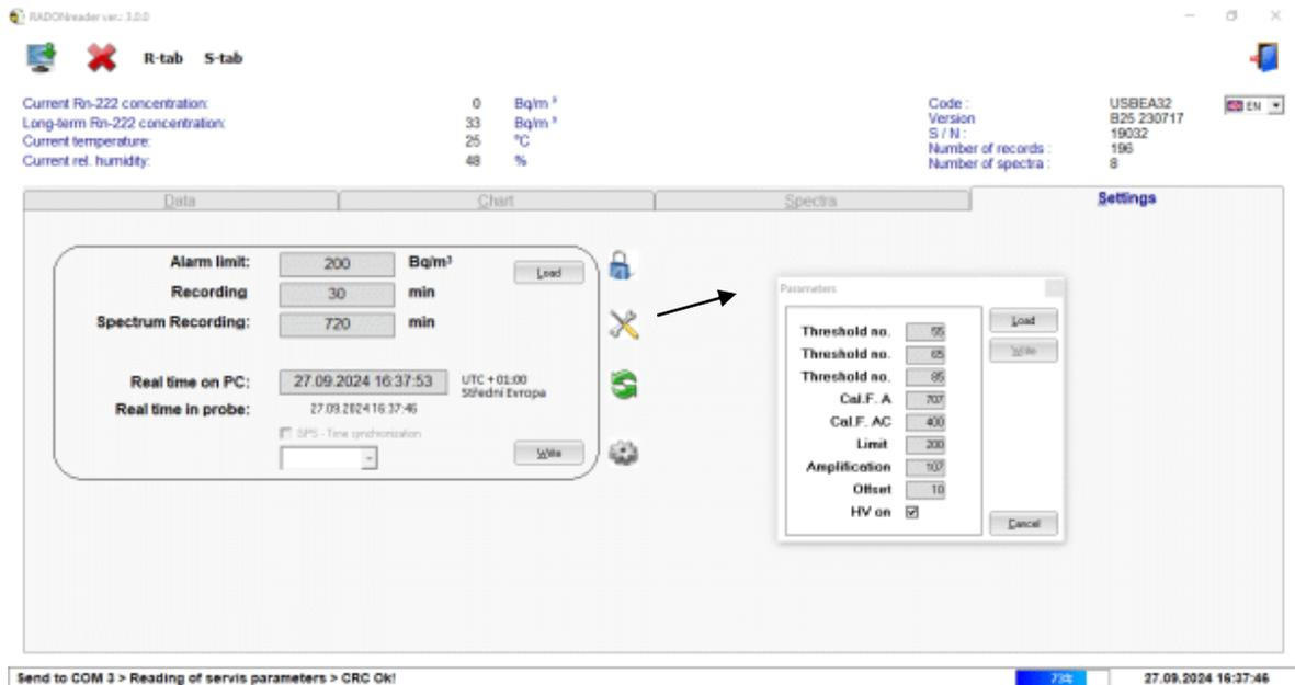
In this tab it is possible to read and change the basic parameters of measurements. To load to settings of the connected probe press „Load“. To upload the current settings from the application into the probe press „Write“. The options in this tab are:
