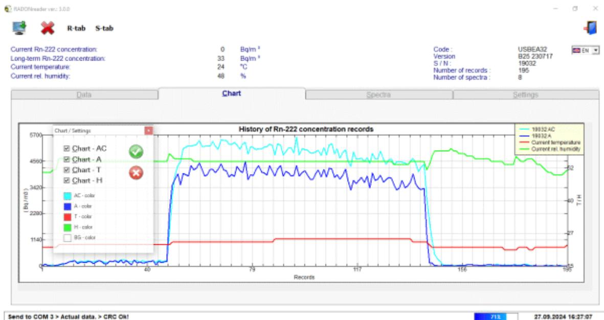
The tab “Chart” shows a figure of radon concentration in time based on the records of short-term/long-term radon concentration (y-axis – radon conc., x-axis – number of measurement). The figure also shows temperature and relative humidity records. The graphs show the same that’s displayed in tab „Data“. For finer control of data plots, we advise to export records and use different plotting software, for example see RadonView in chapter Accessories.
