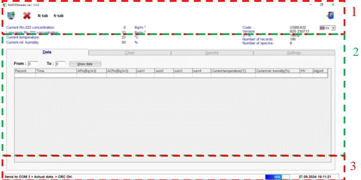
The application opens in one primary window. Secondary windows with additional options may open when pressing some options, for example when pressing the *Exit* button (called *Termination of the program* in the tooltip), a pop-up window will appear asking you if you really want to quit the application. To explain each section of the user interface (UI), it was separated into 3 sections, see picture above.
