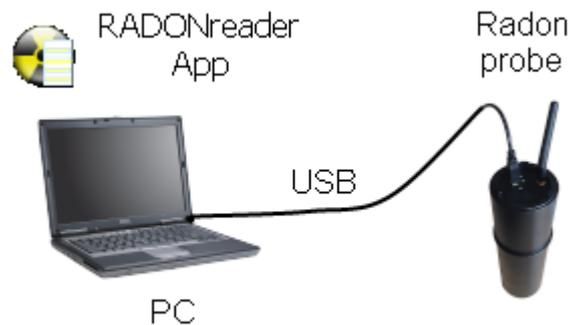
**Figure 1 - Radon Probe connected via USB**
