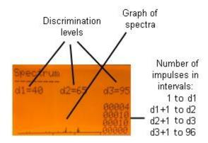
Second graph shows current energy spectrum in array of 96 x 24 pixels and its parameters. Energy spectrum is divide into 96 interval and radon concentration is calculated from intervals d1-d2 (RaA) or from d1-d3 (RaA+RaC). Discriminations d1, d2, d3 are shows below graphs as well.
