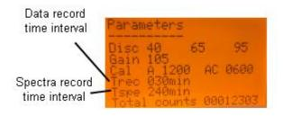
Parameters on third data screen are especially service data but record time intervals are useful.
